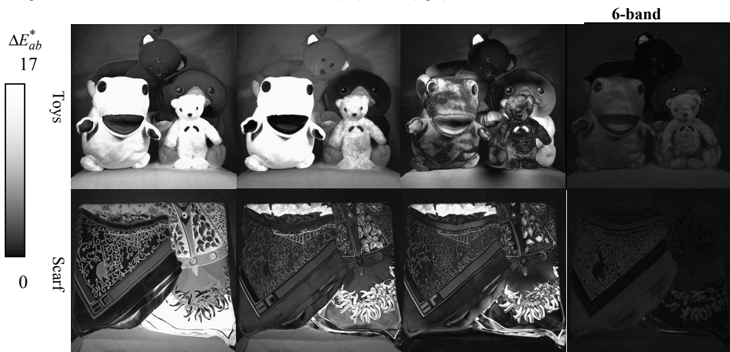
Fig. 10. Visualized \Delta E^*_{ab} image, where 8-bit pixel value corresponds to \Delta E^*_{ab} \times 15 . The upper row is the results of 'Toy' and the lower row is the results of 'Scarf'.
